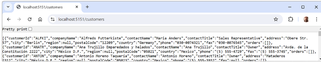
Figure 15.2: Customers from the Northwind database as a JSON document
