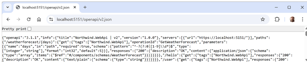
Figure 15.5: OpenAPI JSON documentation for the Northwind web service
